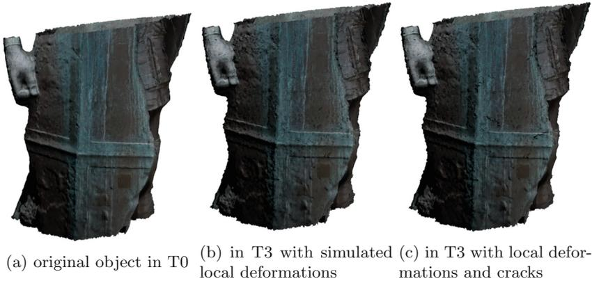
**Fig. 5.** Simulating local deformations and cracks using data from micro-profilometry measurements on sample plates.
